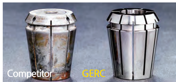
After 4 months Uncoated collet (Left), coated collet (Right)
